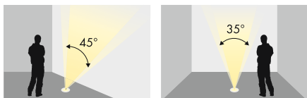
Asymmetrische Linse 45°/35° / Asymmetrical lens 45°/35°
