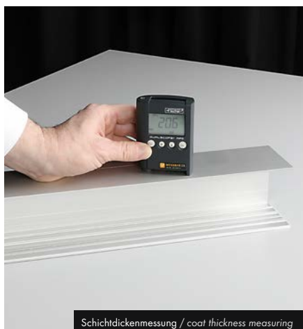
Schichtdickenmessung / coat thickness measuring
